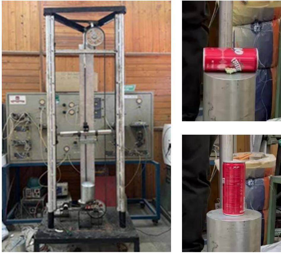
Figure 4: Drop weight impact test setup: (a) Drop weight impact testing apparatus; (b) Drop weight impact tests on aluminum can in (b) Horizontal orientation and (c) Vertical orientation
