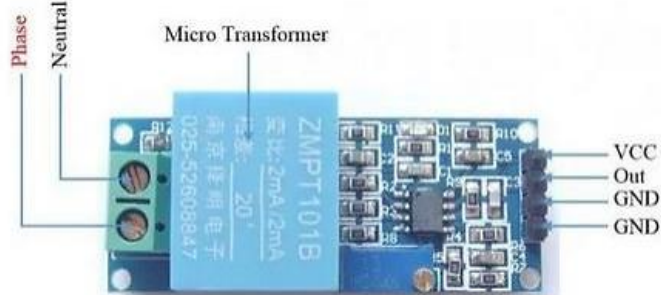
Fig-9: ZMPT101B voltage sensor [41].
