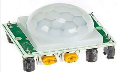
Fig-6: HC-SR501 motion sensor [35].
