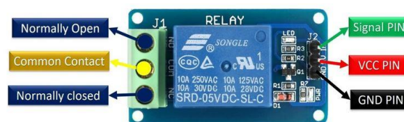
Fig-3: Relay module [30].
