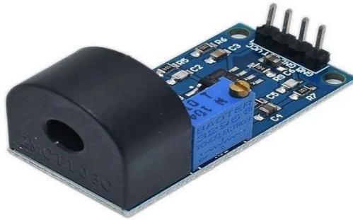
Fig-8: HW670 current sensor [39].
