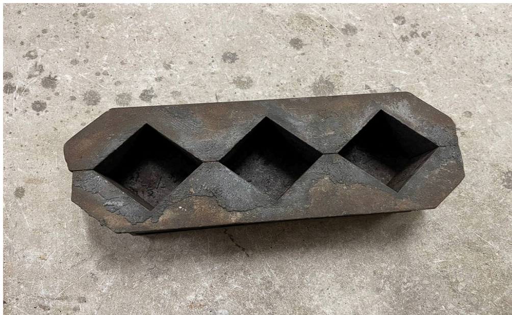
Figure 3.5 :- Prepared Moulds for HSM mix
