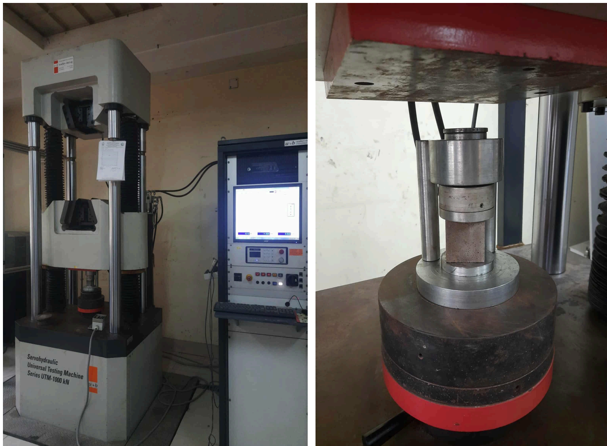
Figure 3.11:- Setup for Compressive Strength testing
