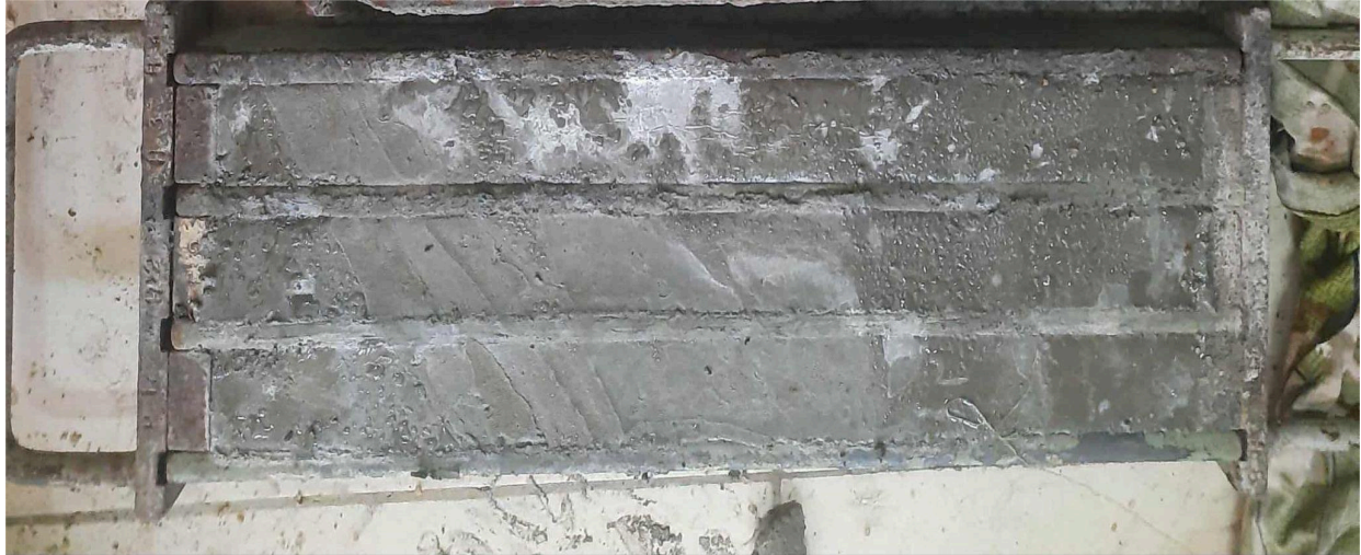
Figure 3.8 :- Moulding of HSM Mix for shrinkage
