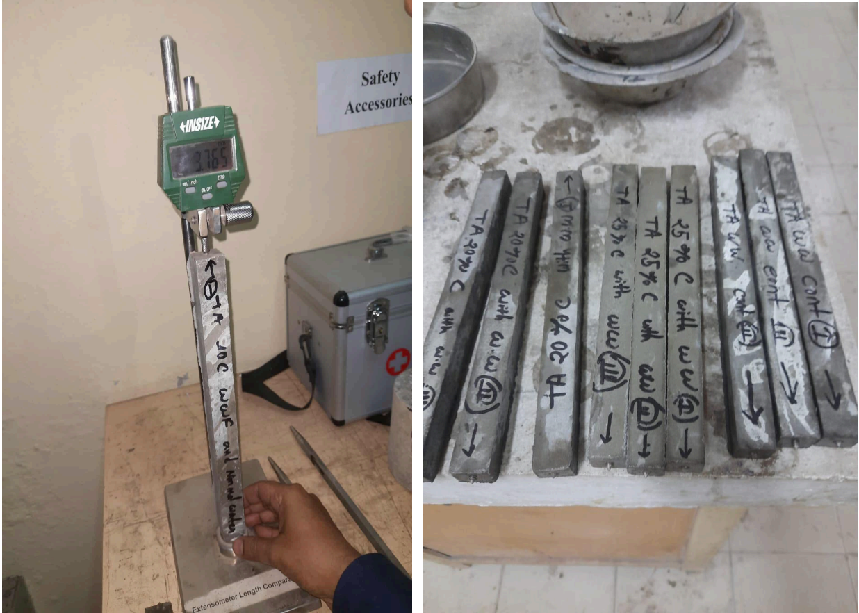
Figure 3.13: Setup for measuring Shrinkage
