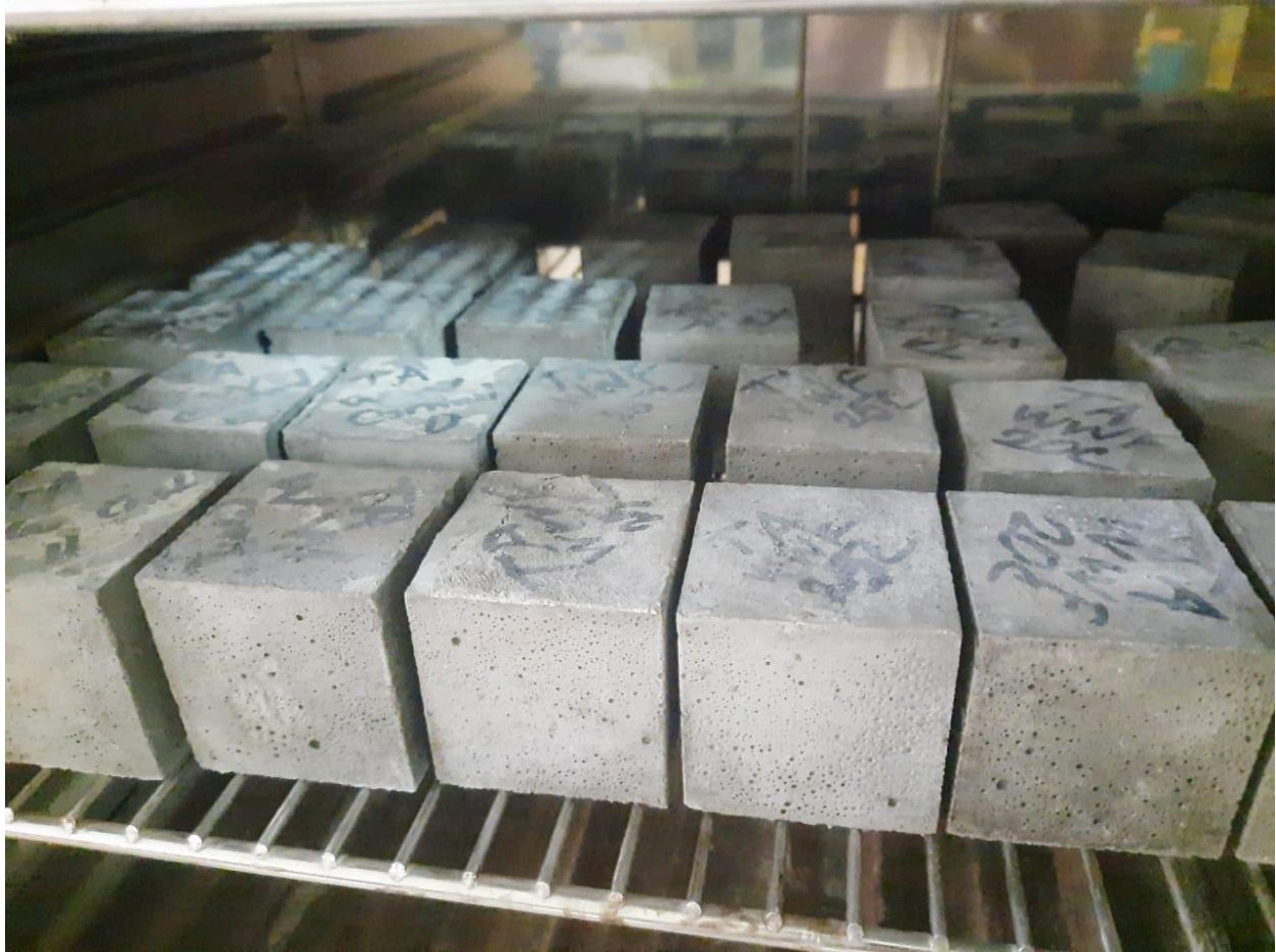
Figure 3.10 :- Increased temperature Curing of Specimens
