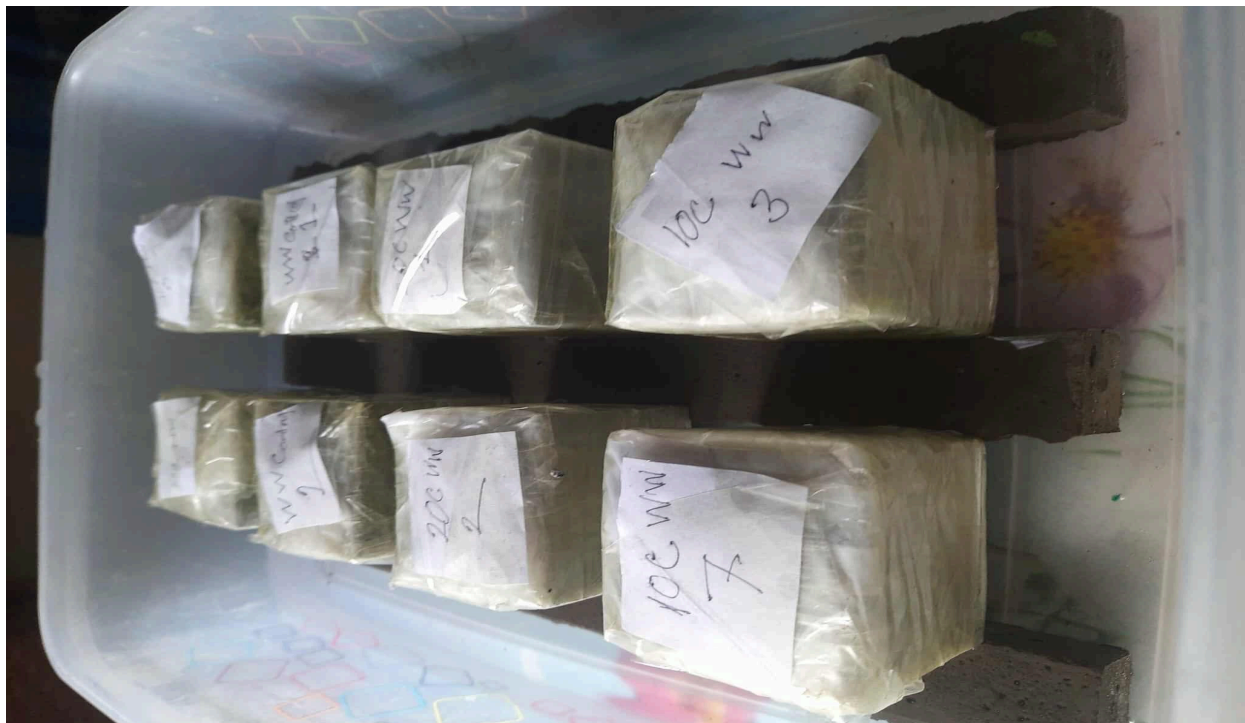
Figure 3.12:- Specimen Setup for Sorptivity Coefficient Measurement as per ASTM 1585- 13
