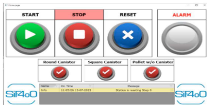
Figure 2.2: Example of a button-based HMI interface in an industrial setting
