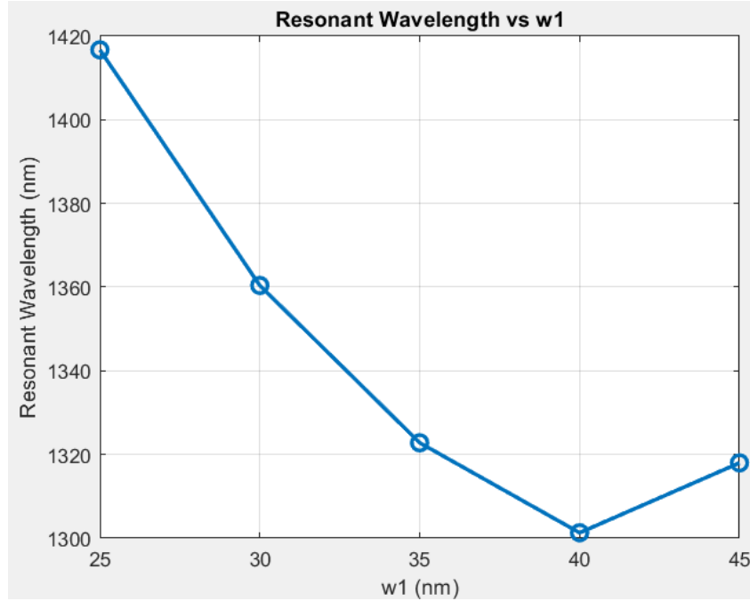
Fig. 4.7 Relation of resonant wavelength with varying w_1
