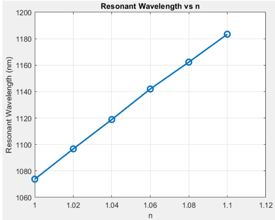
Fig. 3.6 Relation of resonant wavelength with refractive index for mode-2
