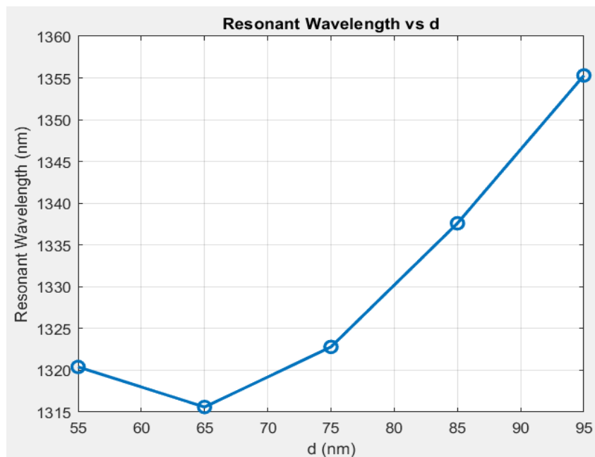
Fig. 4.3 Relation of resonant wavelength with varying d
