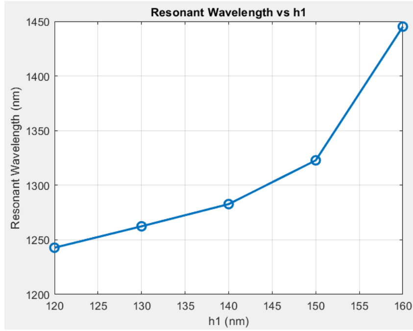
Fig. 4.5 Relation of resonant wavelength with varying h_1
