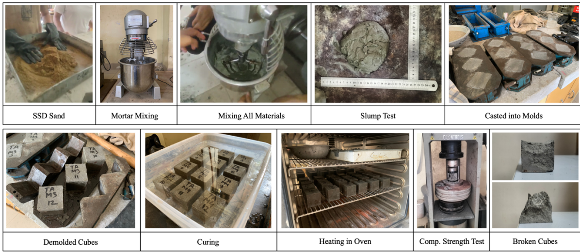
Figure 1: Sample Preparation, Curing and Compressive Strength Test
