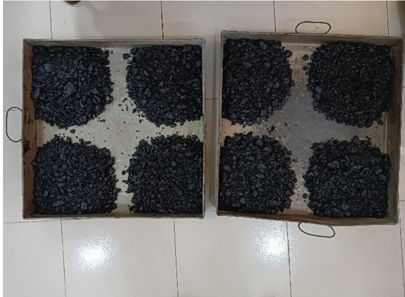
Figure 3. 11 Asphalt loose mixture
