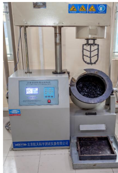
Figure 3. 10 Asphalt concrete Mixture machine
