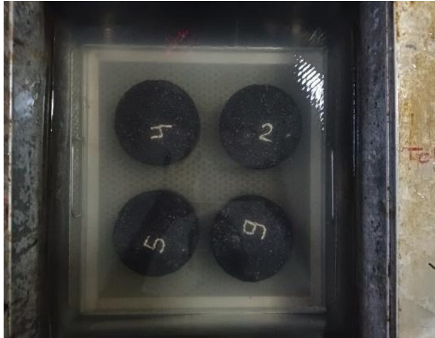
Figure 3. 27 Specimen in 25 0 C water bath
