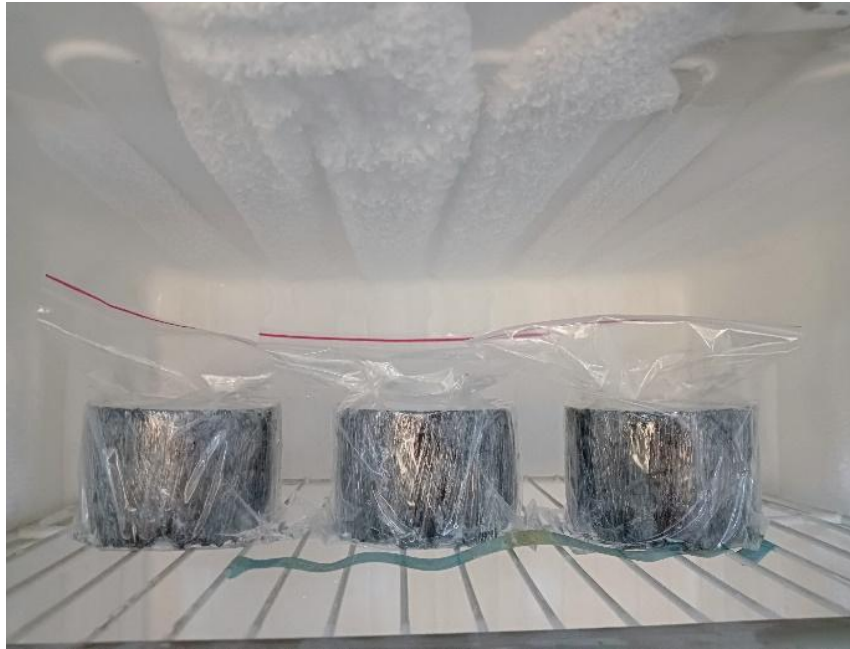
Figure 3. 25 Specimen at -18^{\circ}\text{C} freezer
