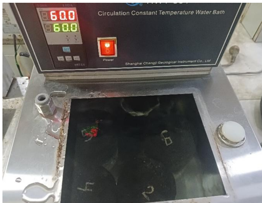
Figure 3. 26 specimen at 60^{\circ}\text{C} water bath
