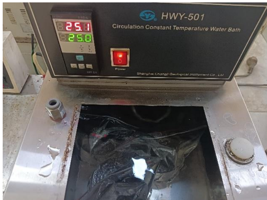
Figure 3. 21 Specimen at 25°C water bath
