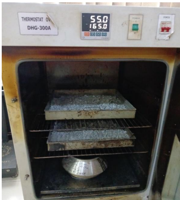
Figure 3. 9 Aggregate and bitumen heated in oven 165^{\circ}\text{C}
