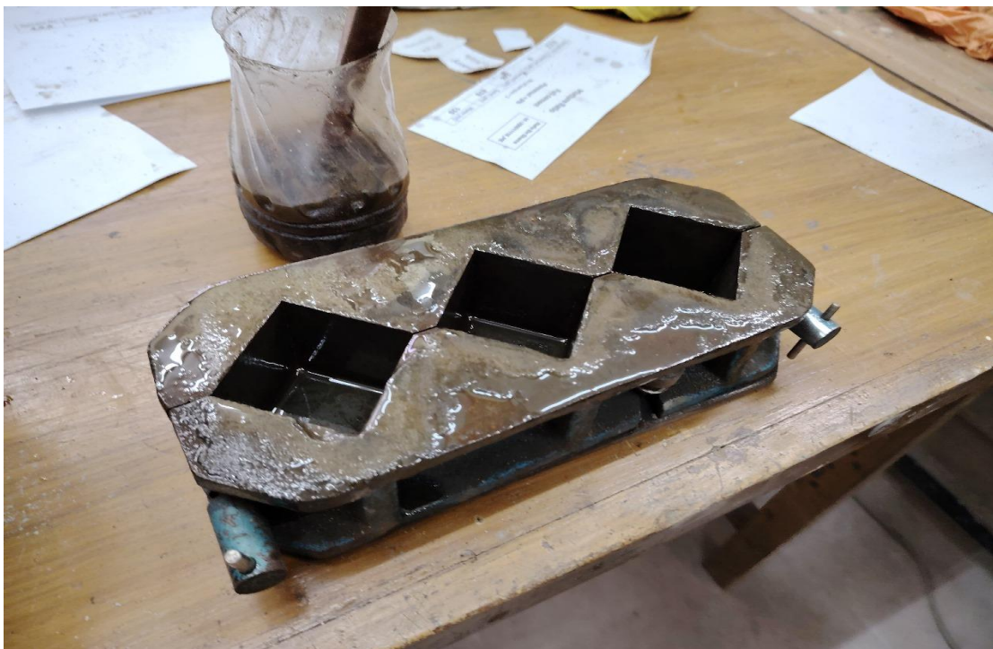
Figure 1 Mold Box Preparation
