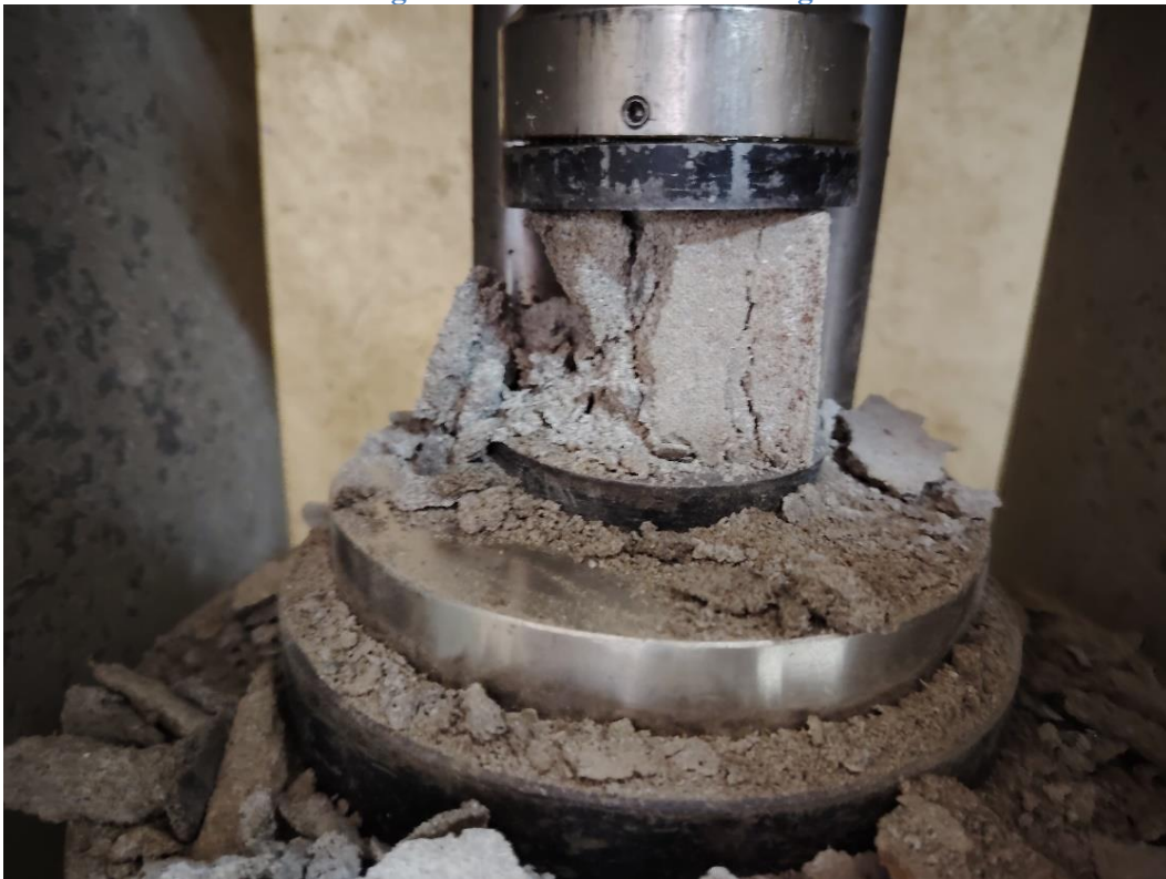
Figure 10 Compression Test of Highest Strength
