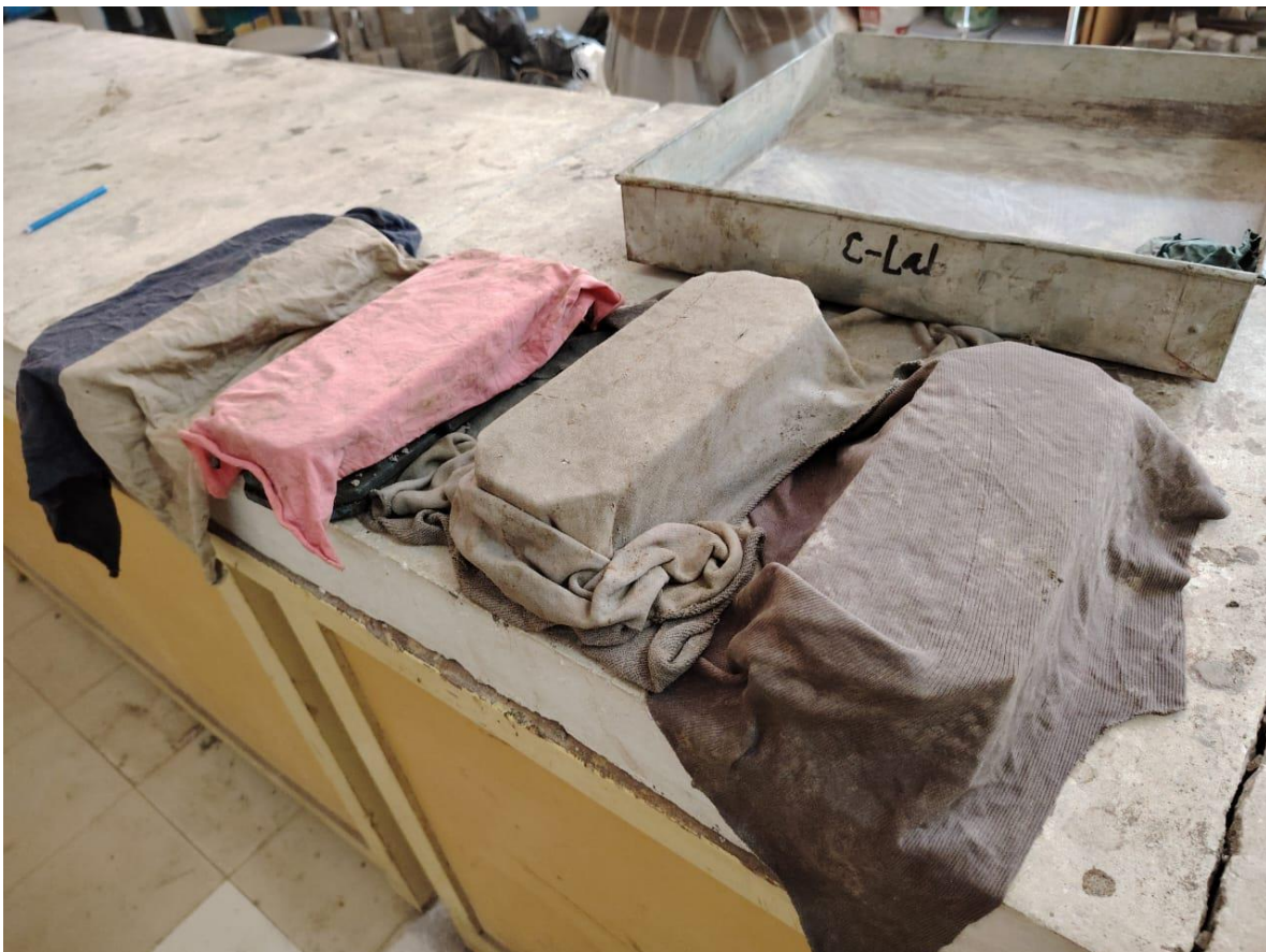
Figure 8 Mold are covered with wet cloth for 24 hours to set
