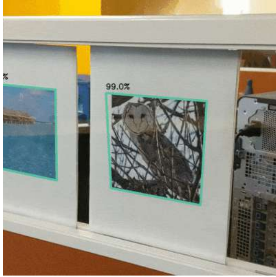
Figure 2.6: Examples of the system in use in natural settings. Message recovery accuracies are shown together with an outline of the StegaStamps that were found and deciphered.
