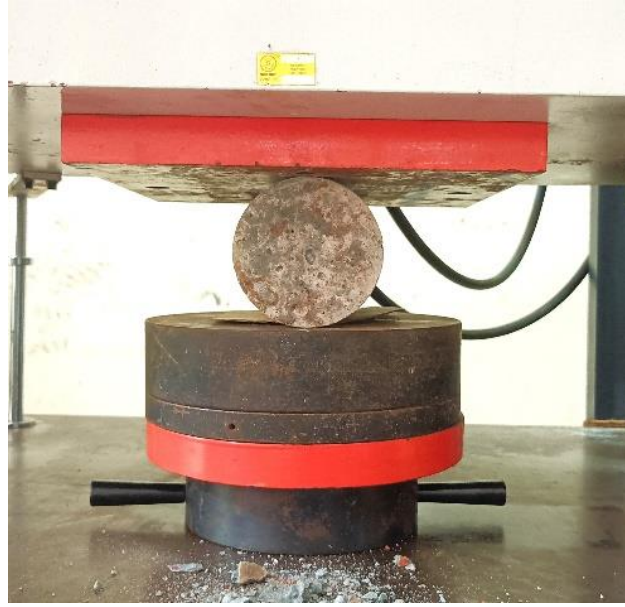
Fig. 3.15: Test setup for splitting tensile strength.
