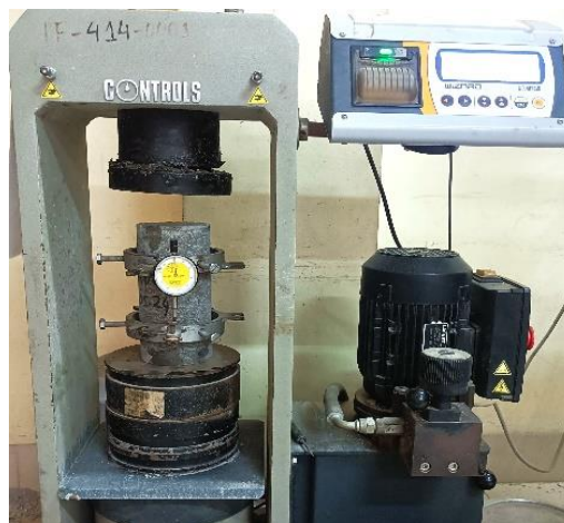
Fig. 3.13: Test setup for compressive strength.
