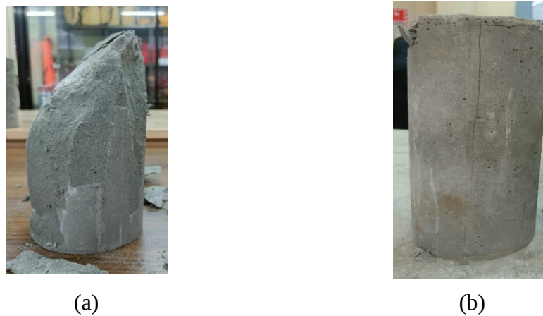
Fig. 4.2: Specimen failure pattern, (a) W/B=0.23 and (b) W/B=0.36
