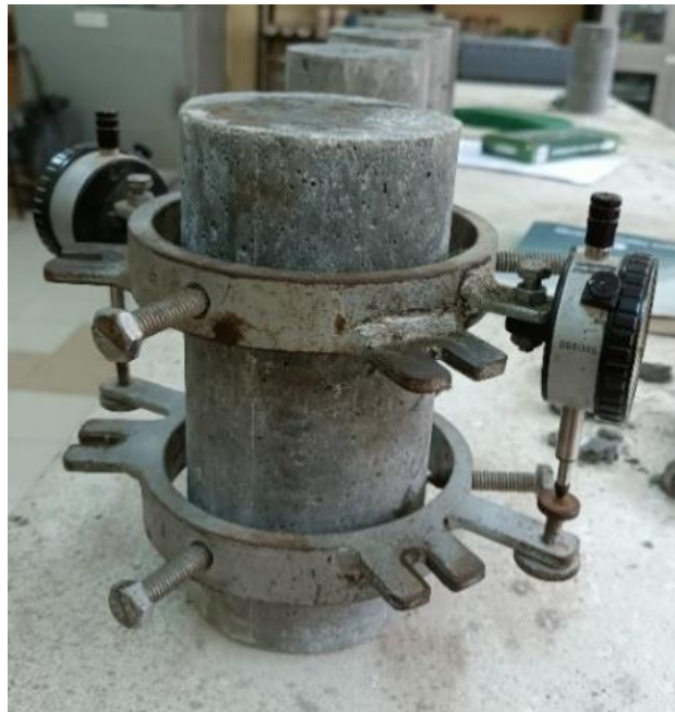
Fig. 3.14: Test setup for strain at peak compressive strength.
