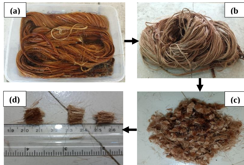
Fig. 3.4: Jute fibre treatment and sizing: (a) fibres in NaOH solution; (b) treated fibres; (c) chopped fibre strands; (d) final 10 mm fibre lengths
