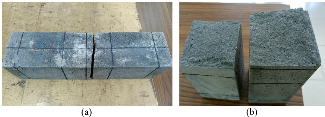
Fig. 5.21: Failure pattern of beam specimen tested under third-point loading.
