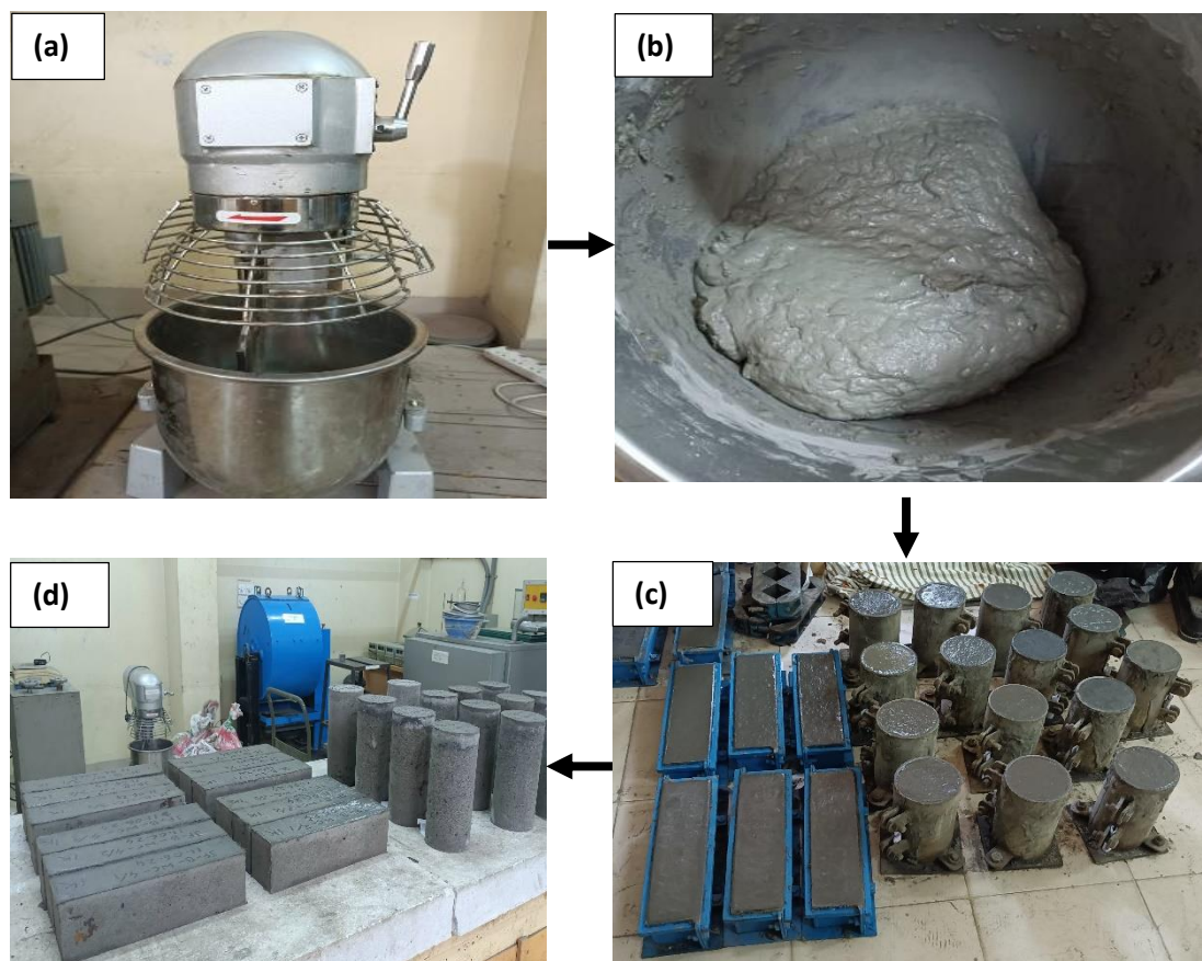
Fig. 3.9: Casting workflow and sample stages: (a) 20 L capacity mixer; (b) freshly mixed composite; (c) fresh mixed composite in steel molds; (d) demolded specimens at 7 days
