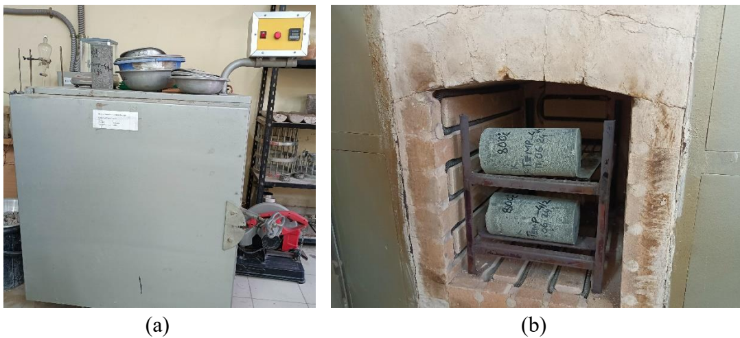
Fig. 5.16: Specimen kept inside an electric furnace
