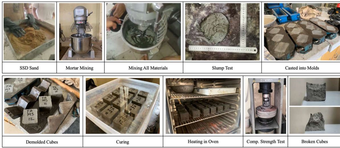
Figure 1: Sample Preparation, Curing and Compressive Strength Test
