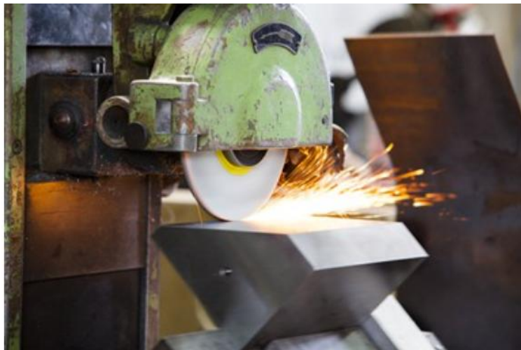
Figure 1.1: Grinding operation (Source: Internet)
