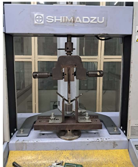
Figure 11: Flexural test setup
