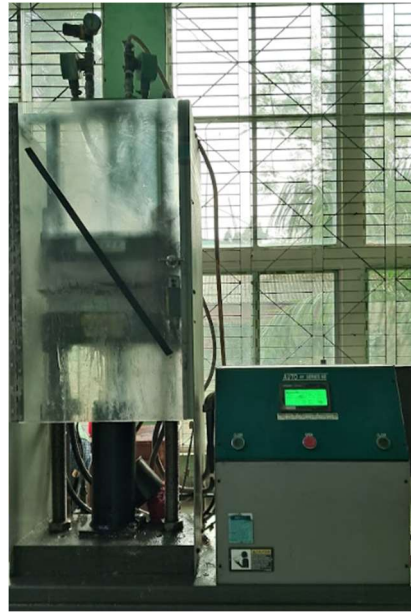
Figure 5: Hot-pressing under 2 MPa pressure at 165°C temperature
