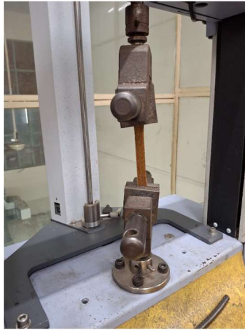
Figure 10: Tensile test setup
