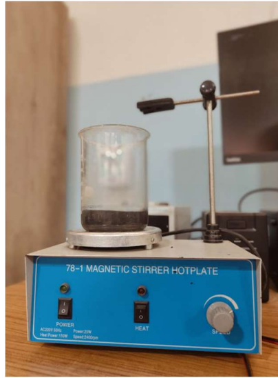
Figure 7: GNP dispersion using magnetic stirrer
